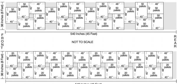
Required Floor Loading Plan for Wood Pallets (PSIN 3919) 540 Inches (45 Feet)
